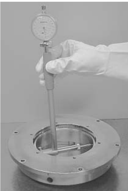
Fig. 1.10 Zero Setting of Cylinder Gauge
