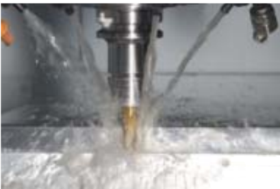
Cutting by NSK Spindle using Ceramic Ball Bearing
