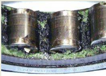
Lubricant degradation caused by electrical discharge currents
